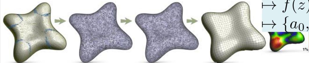
**Figure 1:** A smooth 4-PolyVector field is generated from a sparse set of principal direction constraints (faces in light blue). We optimize the field for conjugacy and use it to guide the generation of a planar-quad mesh. Pseudocolor represents planarity.
