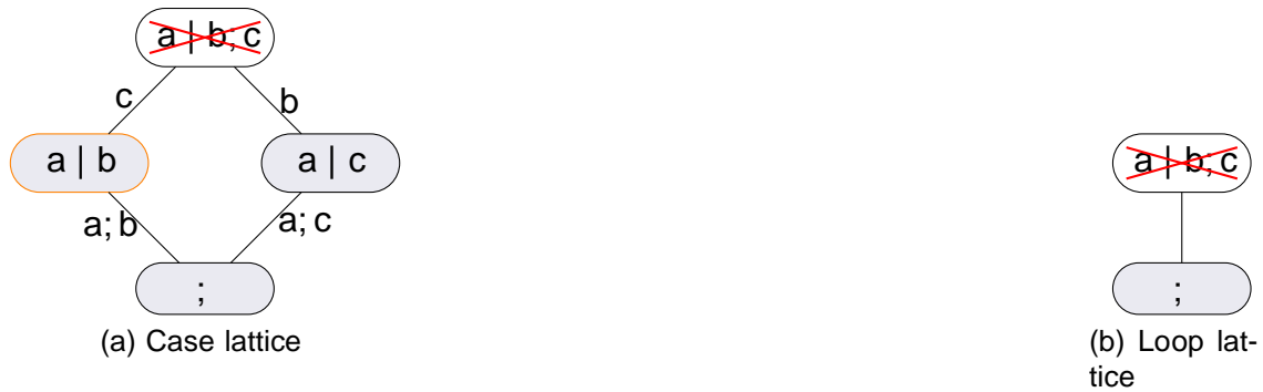
Figure 4-29: This example shows a case and a loop lattice (a \wedge b) \vee (a \wedge c) \vee (a \wedge b \wedge c) . The highlighted lattice point denotes a special region. The code generator only needs to generate a loop over a , so when generating loops it is fine to use the lattice in (b). However, if attempting to generate cases within the loops using the lattice (b), the code generator lacks information saying it needs to perform a different computation in the highlighted lattice point. It also has no way of knowing that it should not compute when a and c have defined values but not when all of a , b and c are defined. The case lattice in (a) contains all of this information and therefore this is the lattice that will be given to the code generator as input.
