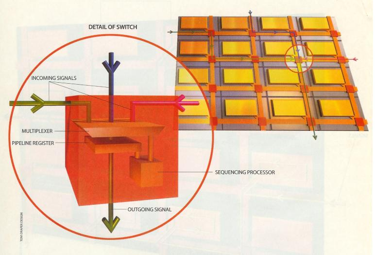
MULTIPLEXING improves the performance of the Raw microprocessor by routing several signals along a single wire segment. The software compiler programs the chip so that the signals converge at one switch in the array of tiles (*right*). The switch contains a multiplexer and a sequencing processor, which are also programmed by the compiler (*left*). Depending on the needs of the application running on the chip, the multiplexer selects one of
