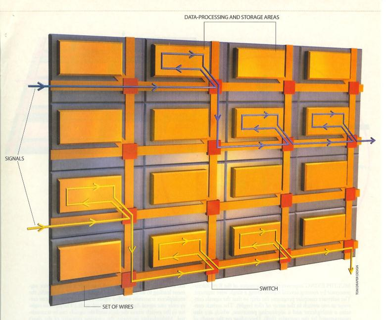
RAW MICROPROCESSOR is a rectangular array of many identical tiles. (Only a small portion of the microchip is shown above.) Each tile contains memory locations that store data and function units where the data are processed. Areas for data processing and storage are represented by the gold rectangles within the tiles. Signals flow through sets of wires that connect each tile to its neighbors. Switches at the wire junctions direct signals to data-processing
