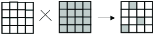
Figure 3: Example crossover operation. White parent is the base parent with a crossover rate of 0.2.
