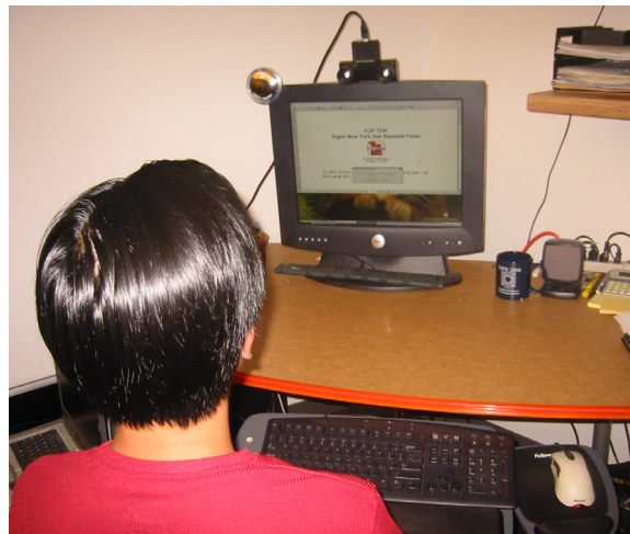
Figure 2: Experimental setup. A stereo camera is placed on top of the screen to track the head position and orientation.
