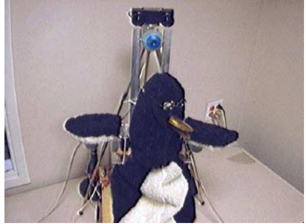
Figure 4: Mel has been developed to study engagement in collaborative conversation[14]. The robot uses information from the stereo camera to estimate head pose and recognize head gesture.
