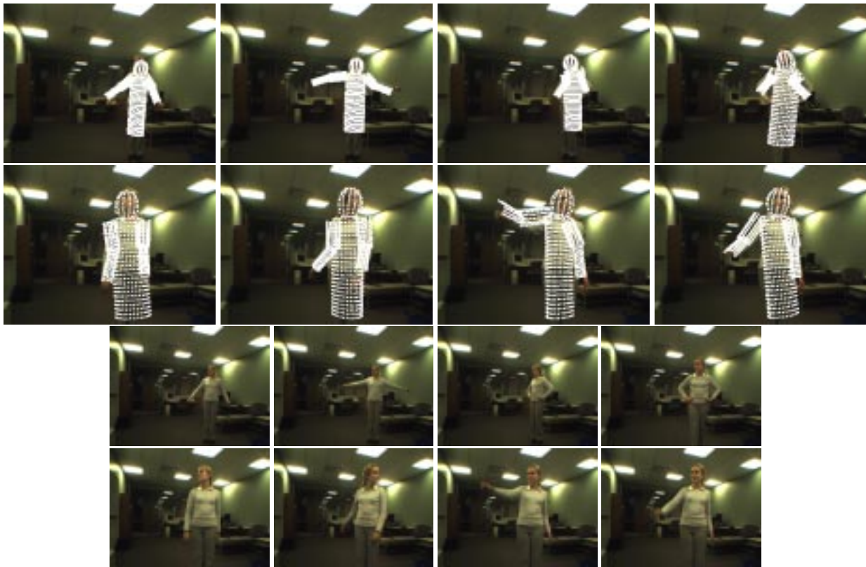
Figure 3: Pointing sequence: Motion capture results. The images show the tracked body poses projected onto the initial images. Image 1 shows the initialization procedure. In the images 3 and 4, we can see that the tracking of the arms of the young girl is not correct. However the tracking algorithm is able to recover from mis-tracking and in the following images, the tracking error has been corrected. In the images 5 and 6, though subtle, we can see that the torso orientation is recovered properly (torso facing right in image 5 and facing left in image 6).
