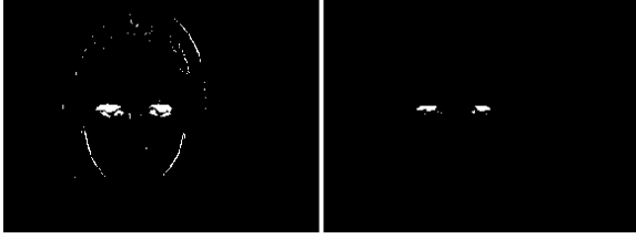
Figure 2: Thresholded difference image prior to erosion (left), and same image after erosion (right). Erosion removes noise caused by insignificant motion in the scene.
