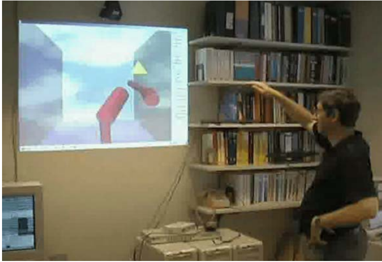
Fig. 3 User interacting with the Virtual Studio application, which allows manipulation of objects with natural gestures and no wires or special markers. A stereo camera (above the projection screen) gives visual information to the tracking system, which estimates the position of the arms of the user (in red on the projection screen) and detects pointed objects (e.g. yellow pyramid).
