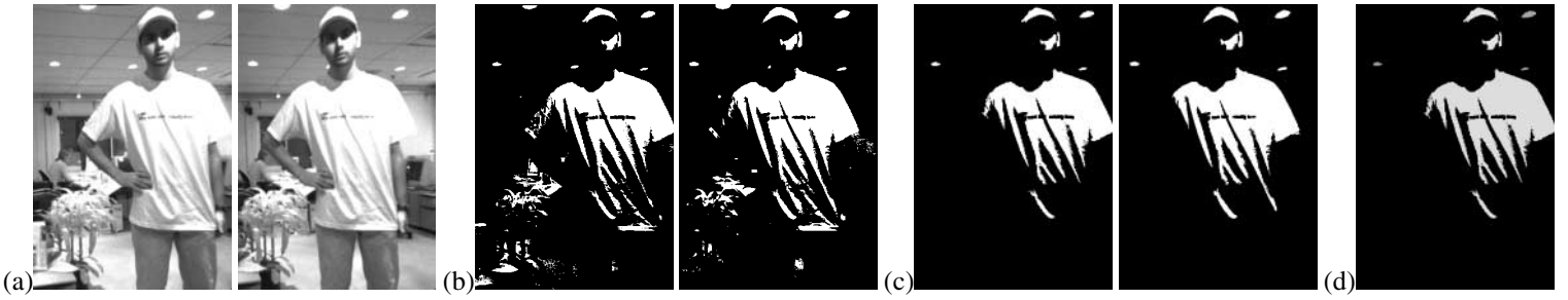
Figure 3: Disparity estimation with uniform planar unoccluded regions. We match a candidate homography between connected components of uniform regions in two views. Unoccluded planes will yield connected component shapes that exactly match according to the given homography. Occluded planes, such as the computer monitor under the user’s arm in the far background, or non-planar objects, such as the plant in the foreground, will not have equivalent shapes and will not be matched. In this example uniform regions were determined by saturated pixels, and the plane was restricted to be fronto-parallel so that image plane translation would determine equivalent matches. (a) shows a stereo pair, (b) saturated pixels in each view, (c) connected components that exactly match in both views for some translation, (d) computed disparity values for each region, shown in grayscale.
