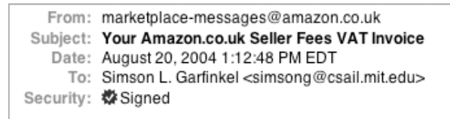
Figure 3. Apple’s OS X Mail application displays a special “Security:” header to indicate if messages are digitally signed.
