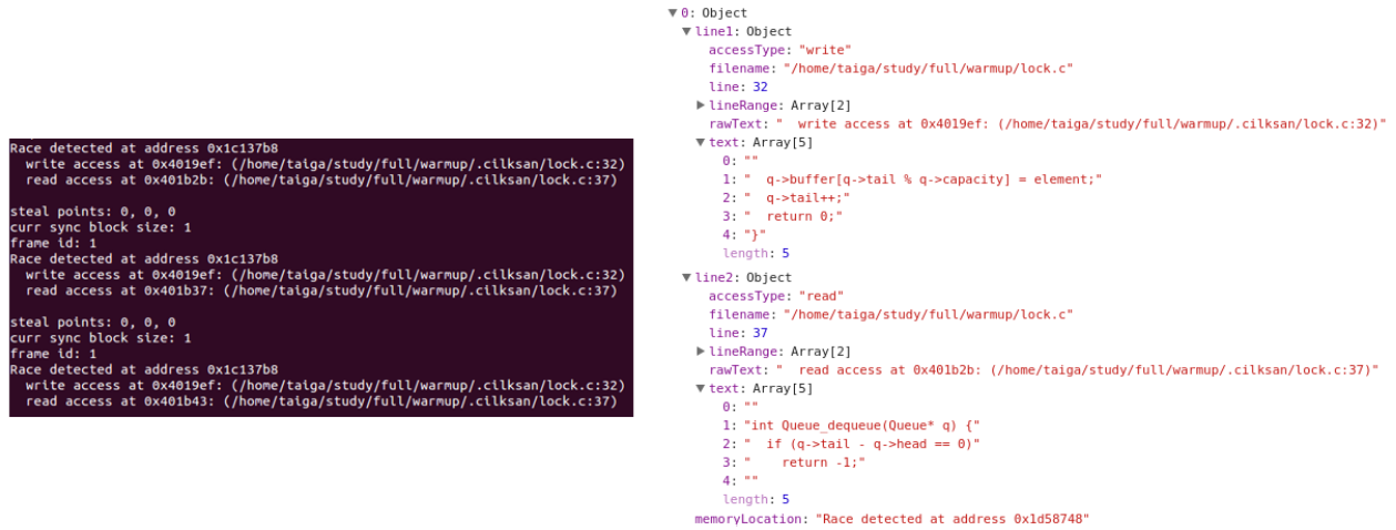
Figure 4-3: Example of the Cilksan parser converting text output to a structured format. The Cilksan parser squashes the 3 race conditions into 1 Object since the 3 race conditions involve the same two lines, and parses out the access type, filenames, and line numbers. It also fetches the racing code, seen in the text field.
