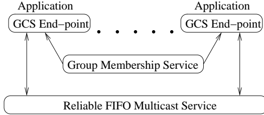
FIG. 4.1. The client-server architecture: GCS end-points using an external membership service. Arrows represent interaction between GCS end-points and underlying services.
