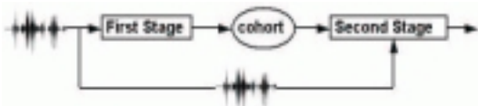
Figure 4: A two-stage speech recognition system. Feature-based models in the first stage generate a high-quality cohort for detailed analysis in the second stage.
