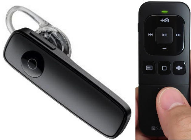
Figure 2-6: Optional accessories for our wearable system. Left: a Bluetooth headset for personal audio. Right: a Bluetooth remote placed within a pocket and used for discreet cueing. All buttons are mapped to a common function so that the wearer need only press against the outside of their pocket.
