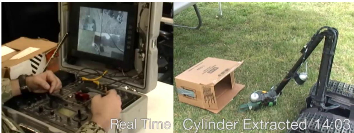
Figure 1.3 Teleoperated Talon robot extracting a cylinder from a box at NAVTECHDIV
