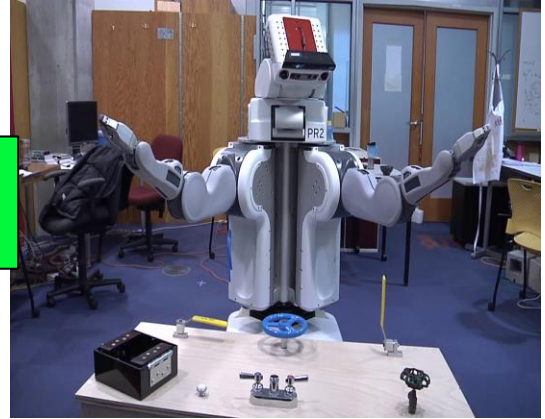
Figure 3.2.1 The surrogate sends RGBD data to the supervisor's 3D, adjustable display.
