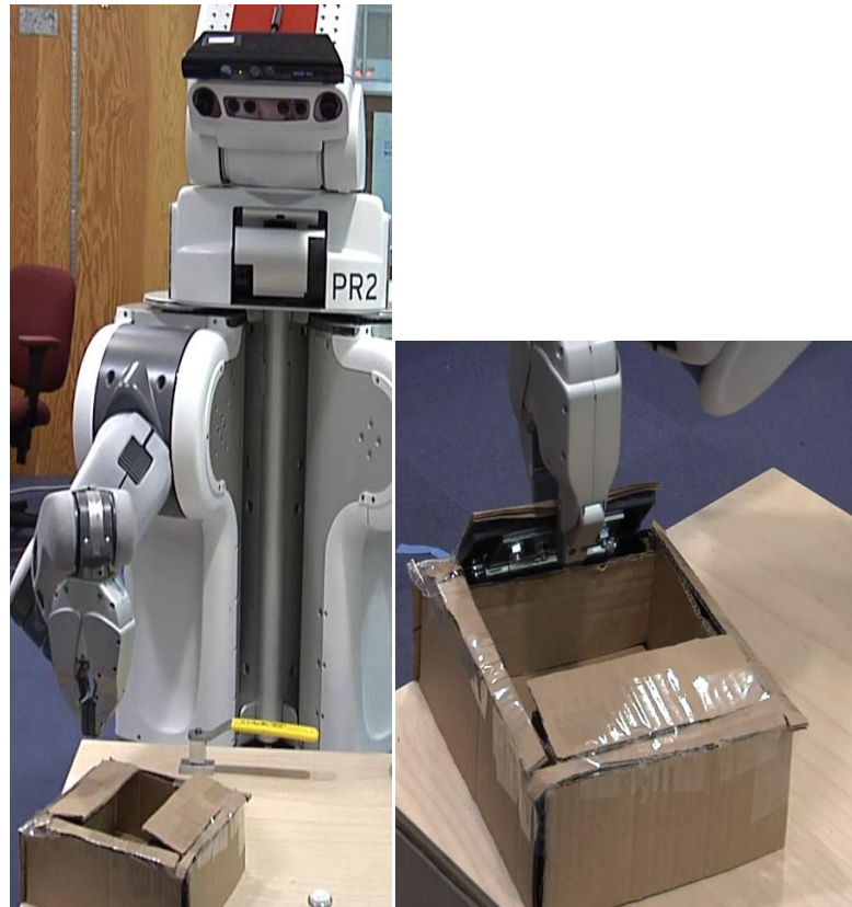
Figure 3.2.9 The surrogate grasps the box flap and opens the box.
