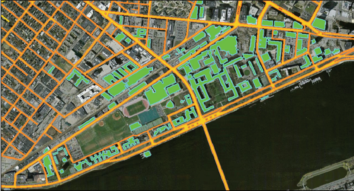
Figure 13. Geometry in a typical GIS is composed of line segments and polygons, often grouped into layers. The key applications of geometry in GIS are the visualization and basic analysis of land use, zoning and various planning functions. Above, geometry of the MIT campus, transformed and projected into the MA state plane coordinate system, is composed mostly of line segments, and some closed polygons.
