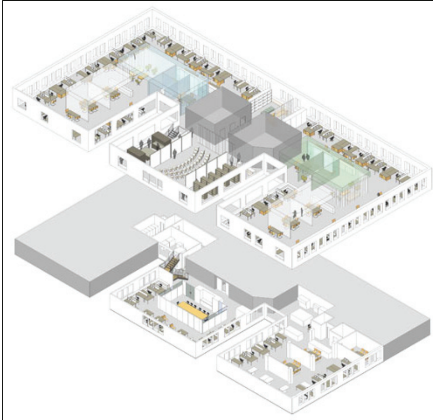
Figure 17. Indoor environments concretely introduce the notion that the xy -plane can be shared by multiple regions. In fact, this is the common case in multi-level building environments. As such, the z -component must in some way be unequivocally represented in order to properly model indoor environments. [Boora2009]
