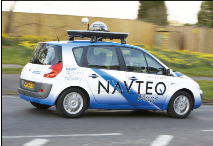
Figure 11. A specially-equipped NAVTEQ car navigates through city streets and acquires massive amounts of raw sensor data. This data is later processed offline and refactored into a commercial GIS dataset product [Symbian2009].
