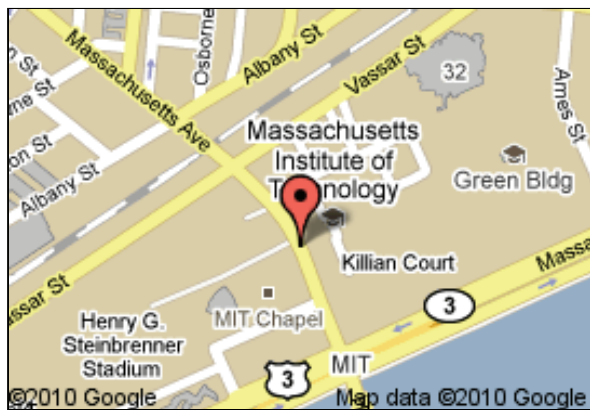
Figure 19. MIT, as a landmark in current GIS, is represented by a single point, in this case its canonical street address: 77 Massachusetts Ave in Cambridge. Enhanced GIS would model landmarks as areas.
