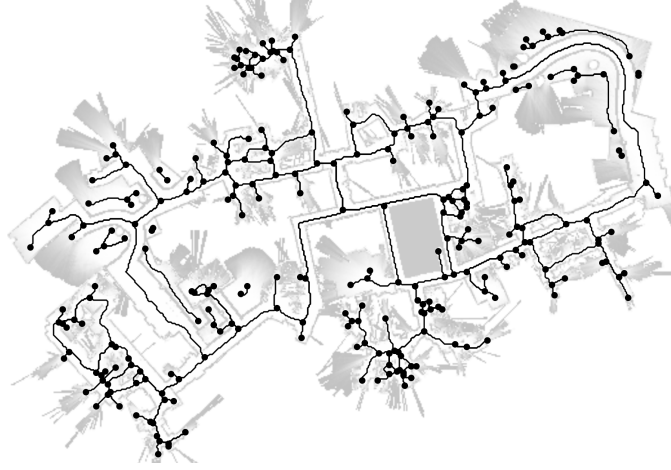
Fig. 4: The automatically generated skeleton of the map, with junction points and end points labeled. We refer to an edge in this graph as a pathlet .
