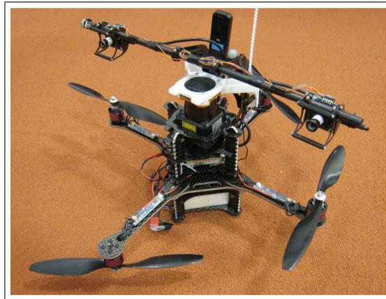
Figure 8. Quadrotor helicopter with Integrated Laser-Stereo Camera
