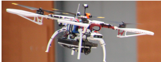
Fig. 1: Quadrotor performing aggressive flight maneuvers autonomously in urban environment. Hardware and sensors include an NUC Skull canyon, an Intel RealSense RGB-D camera and a Flea3 mono camera.
