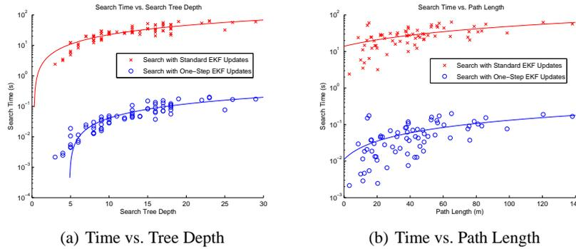
**Figure 3.** Algorithmic Performance. (a) Time to Plan vs. Tree Depth (b) Time to Plan vs. Path Length. Note that these graphs are semi-log graphs, indicating two orders of magnitude increase in speed.
