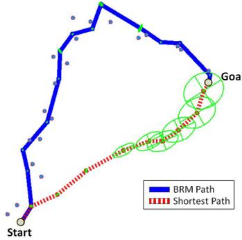
**Figure 1.** Experimental Setup. Range sensor locations (shown as blue circles) were sampled along randomized trajectories between a start and goal location. The solid and dashed line show the plans generated by the BRM and shortest path algorithms, respectively, with green ellipses indicating the covariances  $\Sigma$  along each trajectory. This experimental design tests the ability of the BRM to find paths with greater potential information gain to stay well-localized during execution.
