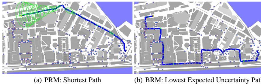
**Figure 4.** Example paths for a mobile robot navigating across MIT campus. The solid blue line in each case is the robot path, the blue dots are the range beacons being used for localization, and the green ellipses are the covariances  $\Sigma$  of the robot position estimate along its trajectory. Notice that the shortest path trajectory grows very uncertain, whereas the lowest expected uncertainty path always stays well-localized at the cost of being slightly longer.
