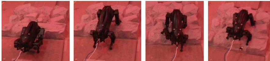
Fig. 8. LittleDog using a dynamic lunge to get onto elevated rough terrain.
