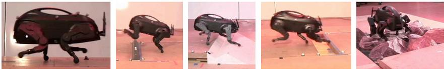
**Fig. 5.** LittleDog traversing various terrain dynamically.
