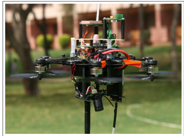
Fig. 3. Our six-rotor helicopter. The helicopter is 29cm in diameter and weighs 142g without the navigation electronics, camera or communication hardware.
