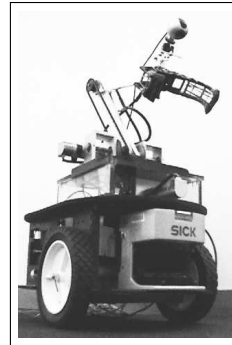
Fig. 16. Our mobile manipulator with a two link arm and gripper. We use a simple webcam mounted on the gripper to capture images of the objects in front of the robot.
