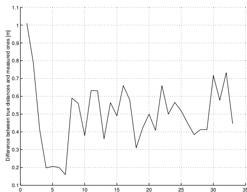
Fig. 2. Difference in metres between the measured and true ranges for the 33 corridor locations.
