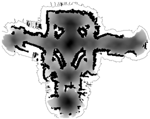
Figure 2: An example map of the entropy, or information content, of the National Museum of American History. The darker an area is, the less information content it contains. The blackest areas of the map are the walls.
