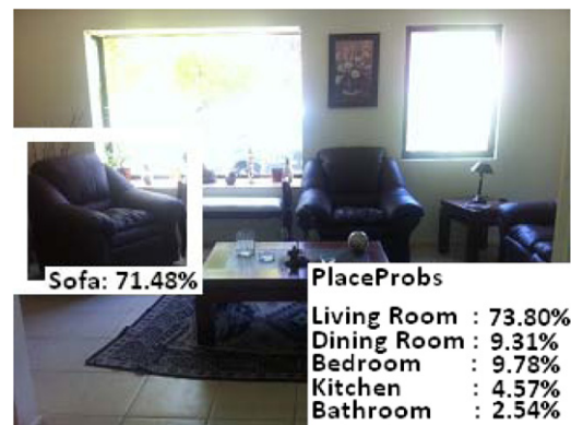
Fig. 14. A Sofa detected in a Living Room, but seeing when the robot is actually in a Dining Room. This produces an error in the scene recognition.
