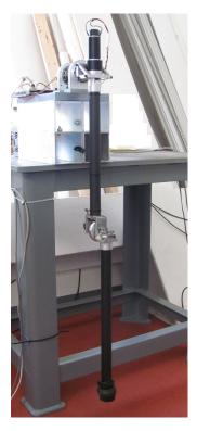
Fig. 1. The "Acrobot" used for hardware experiments.
