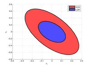
(c)  $\theta_2 - \theta_1$  projection of set of initial conditions,  $B_{\rho(0)}$ , driven to goal set by SOS controller (red) compared to corresponding set for the LQR controller (blue)
