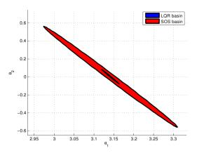
Fig. 2. A comparison of the guaranteed basins of attraction for the time-invariant LQR controller (blue) and the cubic SOS controller (red) designed for balancing the Acrobot in the upright position.
