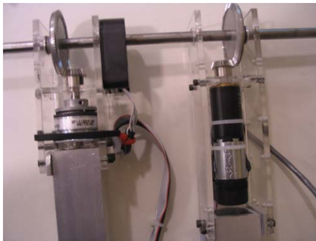
Figure 2-4: Hip Clutch Mechanism. The clutch is adapted to a hip joint to mimic the simple walker with the ability to control the torque and angle between the legs.
