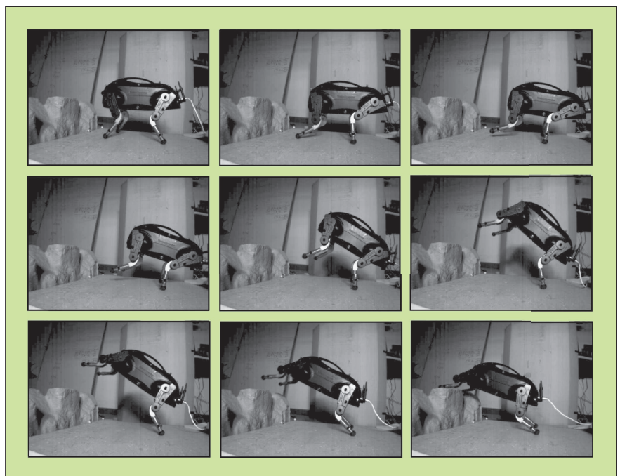
Figure 1. Dynamic behaviors like this jumping maneuver for LittleDog are being developed using reinforcement learning by a team at MIT led by TC chairs Russ Tedrake and Nick Roy. Used with permission from Russ Tedrake.
