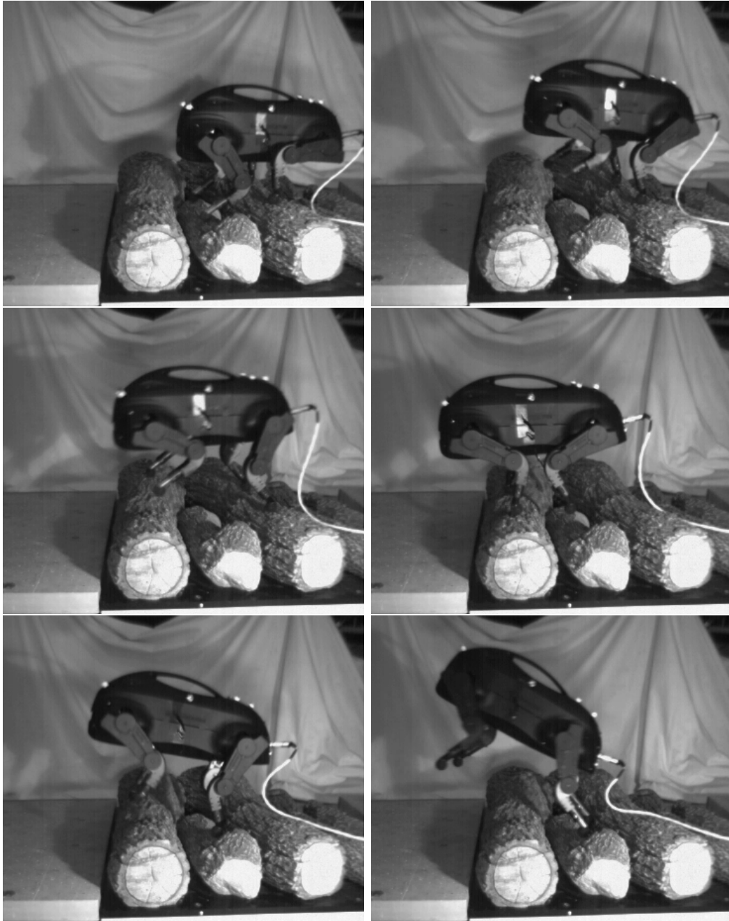
Figure 6-6: Open-loop bounding over logs with LittleDog
