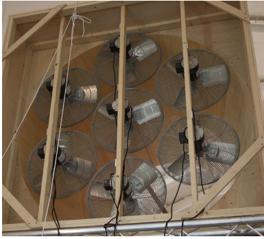
Fig. 10. Rear view of the wind tunnel used for powering the Turbot.
