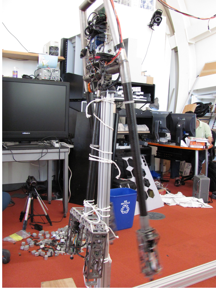
Figure 4-4: The robot with one of the legs fixed, producing a stable configuration and focusing on a subset of the system’s dynamics.
