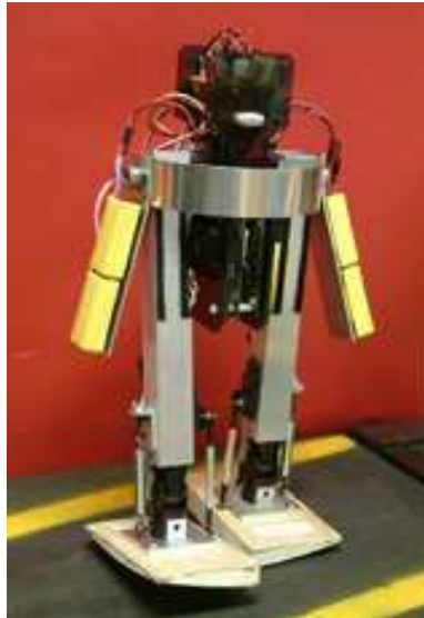
Figure 2-5: Toddler, a 3D biped with optimal control
