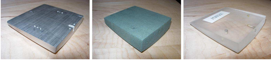
Figure 3-5: Alternate foot materials rejected during production of Passive Toy. Materials (from left to right) include aluminum, rapid prototyping foam, and acrylic.
