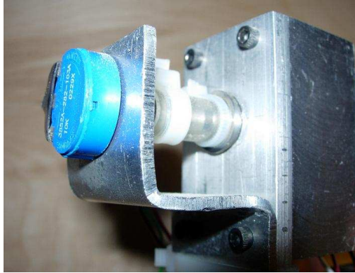
Figure 4-2: Potentiometer mounted on hip joint of Toddler used to measure hip angle.
