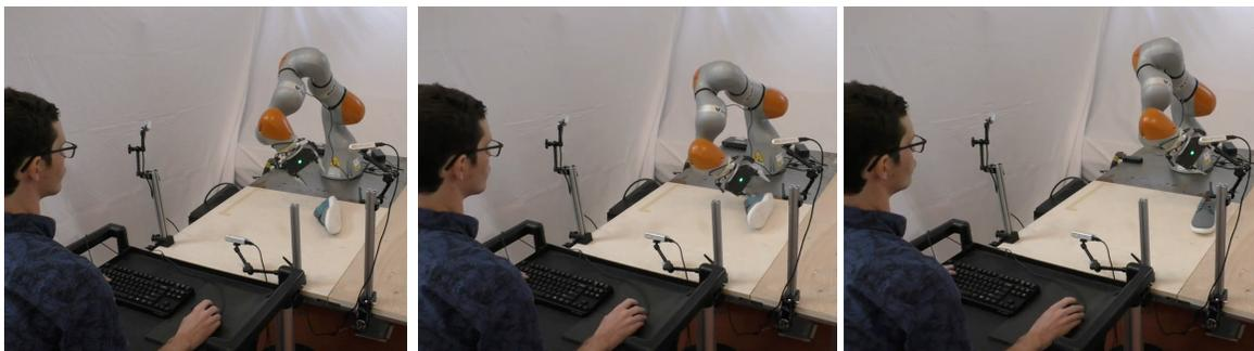
**Figure 5-4:** Example demonstration, in this case for the shoe flip task, with the robot teleoperated by the demonstrator.
