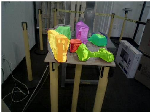
**Figure 2-4:** Example segmentation performance (alpha-blended with RGB image) of network ( $e$ ) on a multi-object test scene.
