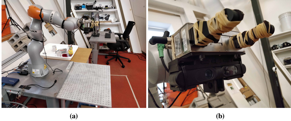
Figure 7: (a) Kuka IIWA LRB robot arm. (b) Schunk WSG 50 gripper with Primesense Carmine 1.09 attached
