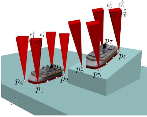
Fig. 2: The linearized friction cones at each corner of the feet.
