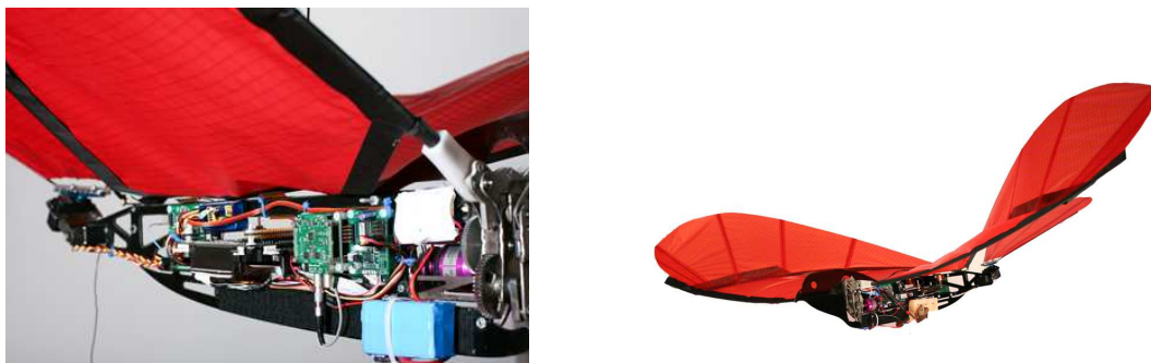
Figure 6-2: Our initial design of a fully instrumented computerized ornithopter. The robot has a 2m wingspan and is capable of carrying a 440g instrumentation payload. Design by Zack Jackowski.
