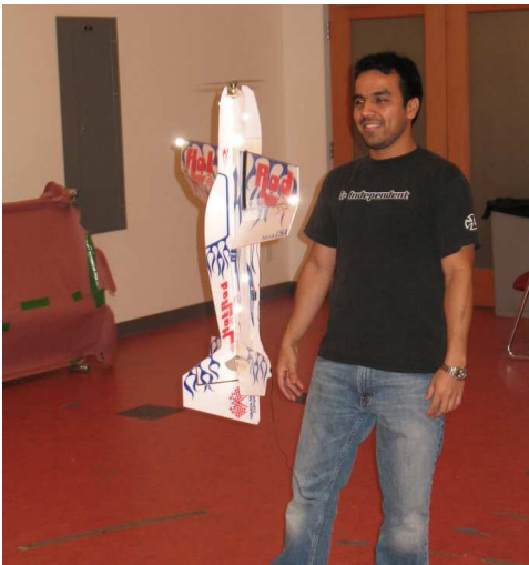
Figure 1-1: Autonomous Vertical hover (prop-hang). This maneuver was executed using simple PD control.
