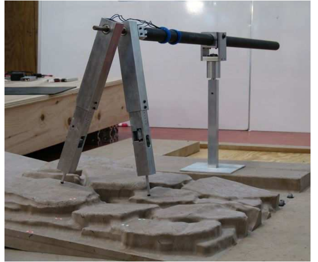
Fig. 25. Compass gait robot posed on rough terrain.
