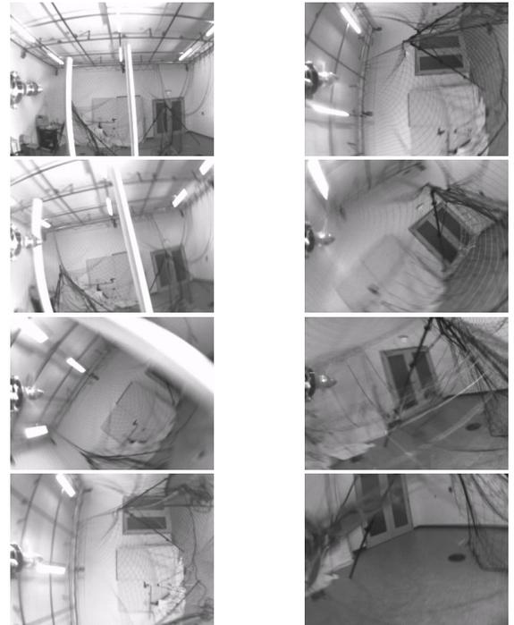
Fig. 11: Sequence of stills from an onboard camera during the knife-edge maneuver. Each image is 0.083 seconds (83ms) after the previous. The entire set captures a total of 0.583 seconds.
