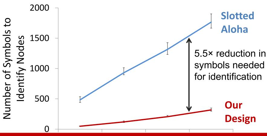
Network compressive sensing improves efficiency of node identification by  $5.5 \times$
