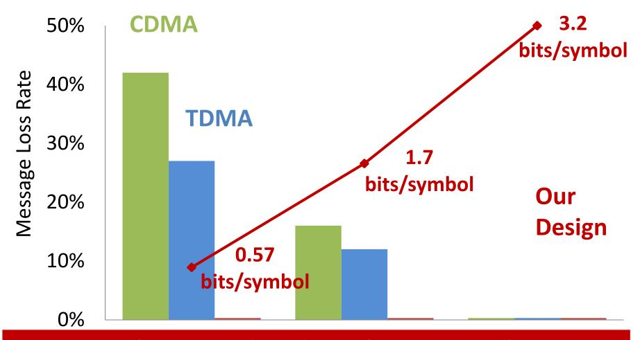
Network as a node adapts bit rate to eliminate message loss
