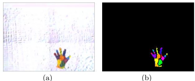
Figure 5: (a) Resultant image after background removal; (b) result of color classification after background removal
