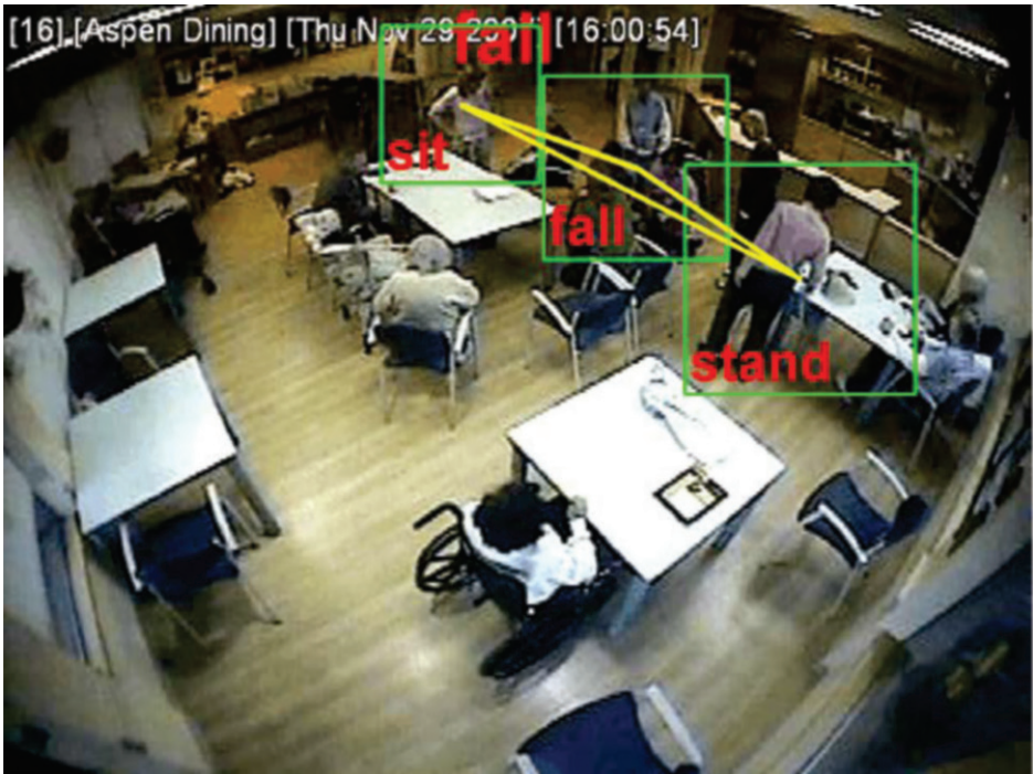
Fig. 6.6: Nursing-home dataset: Samples with some results of fall detection. Image courtesy to G. Mori, SFU for his permission.
