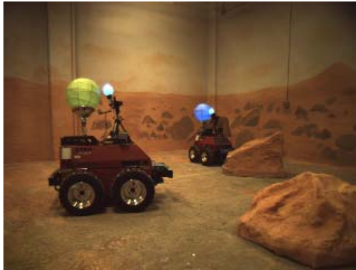
Figure 5-2 Rover Test-Bed used to test STN reformulation algorithms
