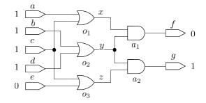
Figure 1. The Boolean Polycell example consists of three OR gates and two AND gates. Input and output values are observed as indicated.
