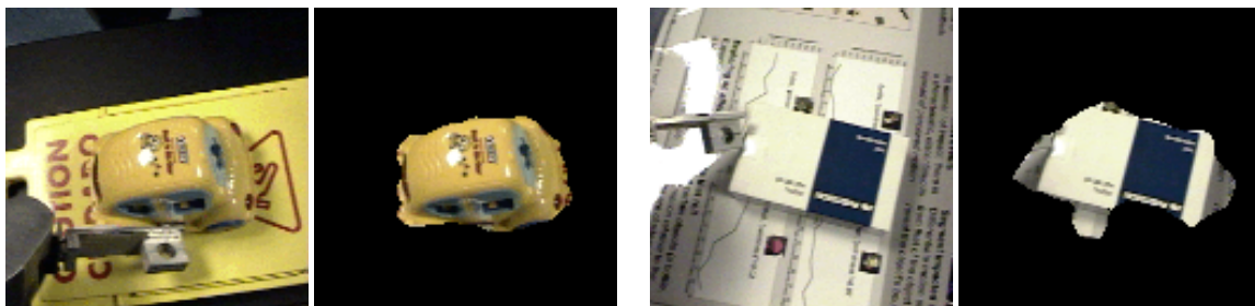
Figure 3-10: Challenging segmentations. The example on the right, a blue and white box on a glossy poster, is particularly difficult since it has complex shadows and reflections, but the algorithm successfully distinguishes both the blue and white part of the box from the background.
