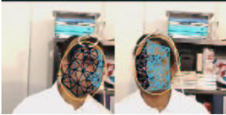
Figure 8-19: A visualization of surface coordinates on the mesh. The mesh has been colored here based on the sign of a surface coordinate, so that it appears as two halves locked onto either side of the face.
