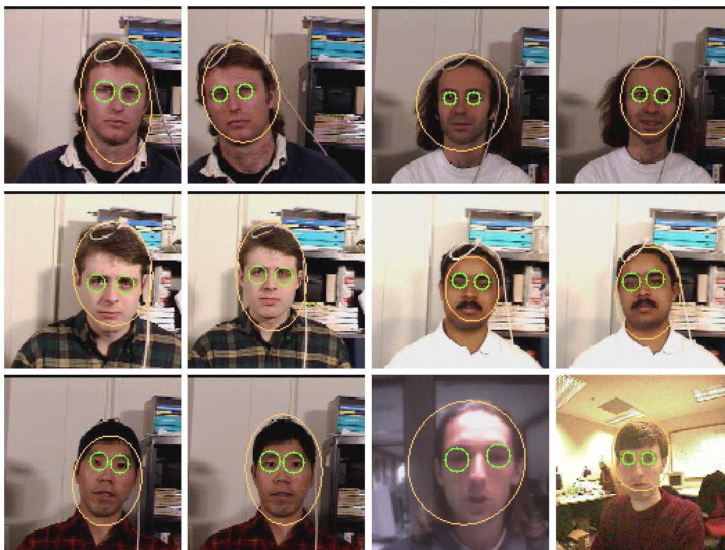
Figure 8-17: Frontal pose being recognized for a number of individuals. As noted in the text, roll of the head is not problematic since it will be parallel to the image plane and so can be recovered directly from the angle the eyes make with the horizontal.
