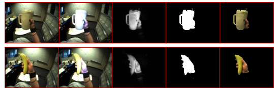
Figure 5: The wearable system currently achieves segmentation by active sensing. When the wearer brings an object up into view (first column), an oscillating light source is activated (second column). The difference between images (third column) is used to compute a mask (fourth column) and segment out the grasped object and the hand from the background via a simple threshold.(fifth column).
