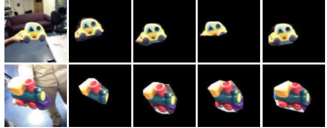
Figure 7: Periodic motion can also be used to segment an object held by the teacher, if they shake it.
