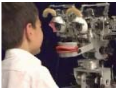
Figure 1: Kismet is an expressive robotic creature designed for natural social interaction with human [1].
