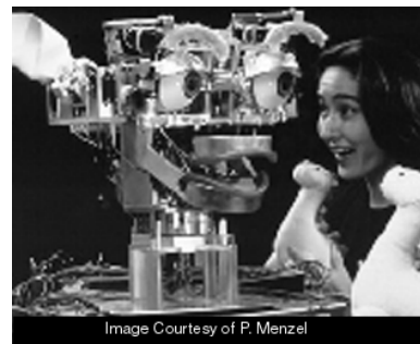
Figure 1. Kismet is an expressive robotic creature designed for natural social interaction with human[1].
